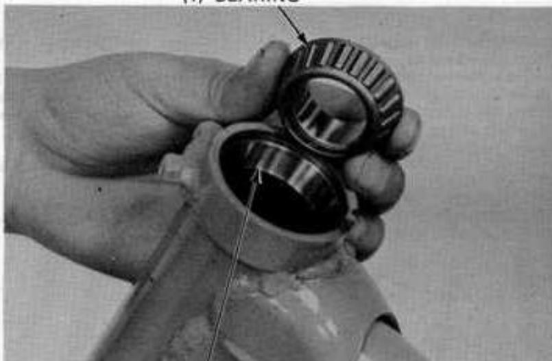
(2) BEARING RACE (1) BEARING RACE REMOVER (07953-MA00000)
