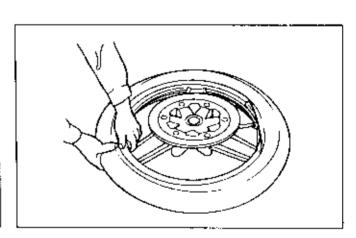
When the remaining bead is only 50 - 60 mm (2 to 2.5 in), pull the two levers up and over.
