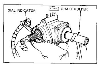
If the difference in measurements exceeds the limit, it indicates that the bearing is not installed squarely. Inspect the bearings and reinstall if necessary.
