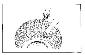
Date of Issue: Sep., 1988 © HONDA MOTOR CO., LTD. Install a rubber plug into the hole as follows:
