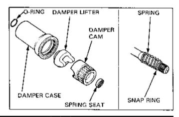
Date of Issue: Sep., 1988 © HONDA MOTOR CO., LTD. Remove the oil seal, oil seal guide and damper spring from the damper case.
