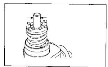
Measure the dam'per spring free length. Replace the spring if the free length exceeds the service limit.
