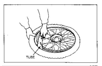
Remove one side of bead using same procedures as the tubeless tire.
