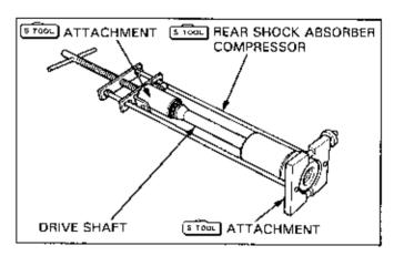
Compress the damper spring and remove the stop ring. Remove the tool.
