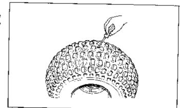
Insert and center a rubber plug through the eye of the inserting needle.
