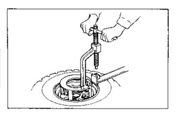
If the bead breaking is difficult with the narrow end (A side) of the breaker arm, use the wide end (B side) of the arm and repeat the procedure in the previous step.
