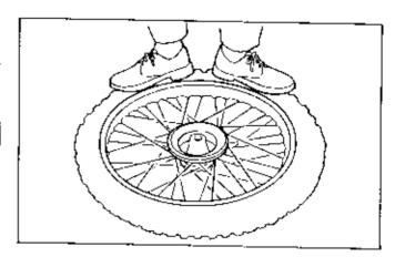
Collapse the bead into the rim center and stide the tire out of position.
