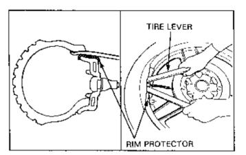
Repeat the above procedures until half of bead is removed. Then remove the remaining bead by hand,
