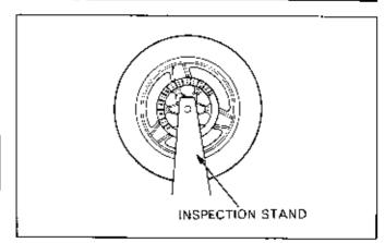
Mount the wheel, tire and brake disc assembly in an inspection stand.
