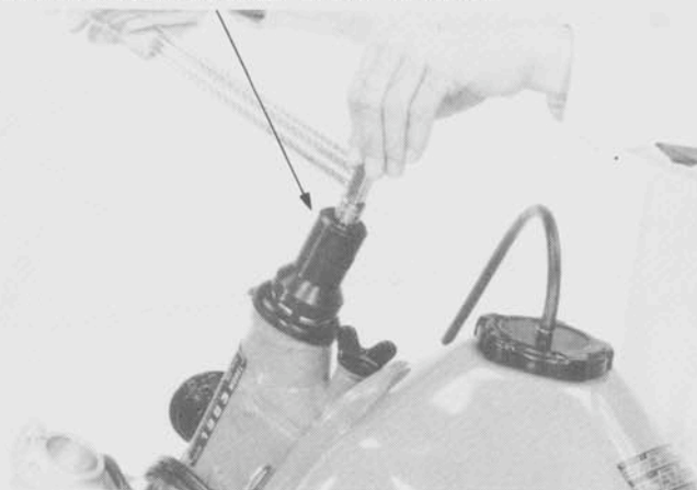
STEERING STEM SOCKET 07916-3710100
