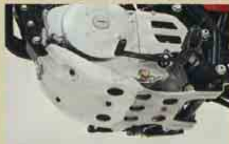
Alloy skid plate helps protect underside of engine and five-speed transmission.
