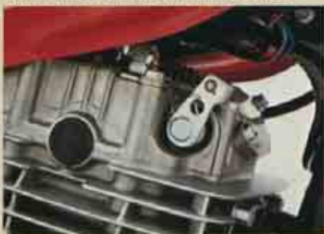
Automatic compression release opens exhaust valve to reduce kickstart effort.
